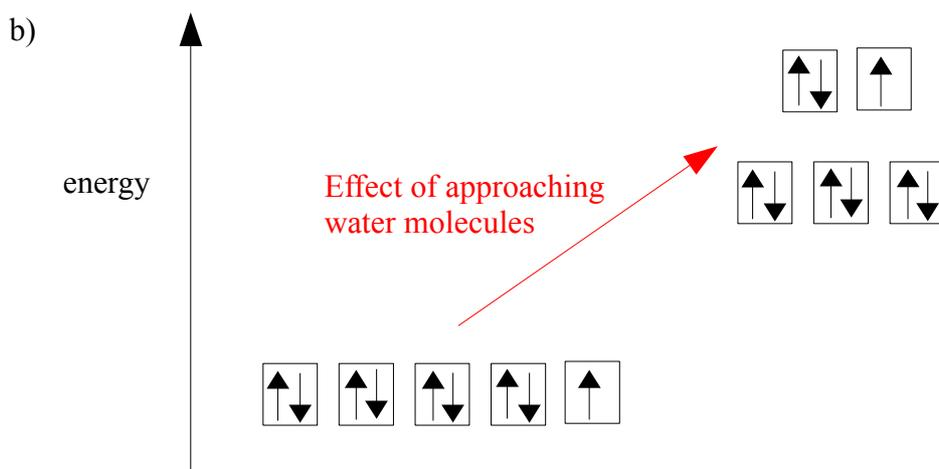
c) The water molecules increase the energy of all the d orbitals, but there is now an energy gap within the d orbitals, with two of the orbitals having a higher energy than the other three. If light of the right frequency (and therefore energy) falls on the ion, an electron from the lower energy orbitals can be promoted into the space in the higher energy orbital.
